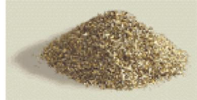
Redox is simply the principle of opposites at work. When contaminants in water come in contact with redox media, some lose electrons to the media while others gain electrons. This gain or loss of electrons changes the chemical nature of the substance.
